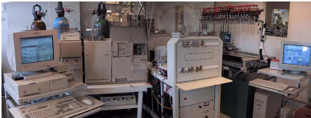
Figure 1 Photograph of the EA/IRMS/CT (from left to right) system, employed for combustion of organic samples for the Groningen AMS facility
