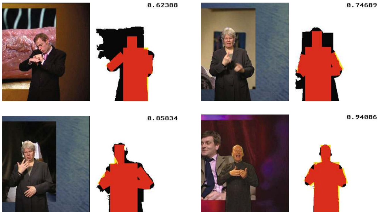
Fig. 8 Examples of frames with different segmentation overlap scores. The masks show the segmentation (black), rendered silhouette (yellow) and their intersection (red) (Color figure online)
