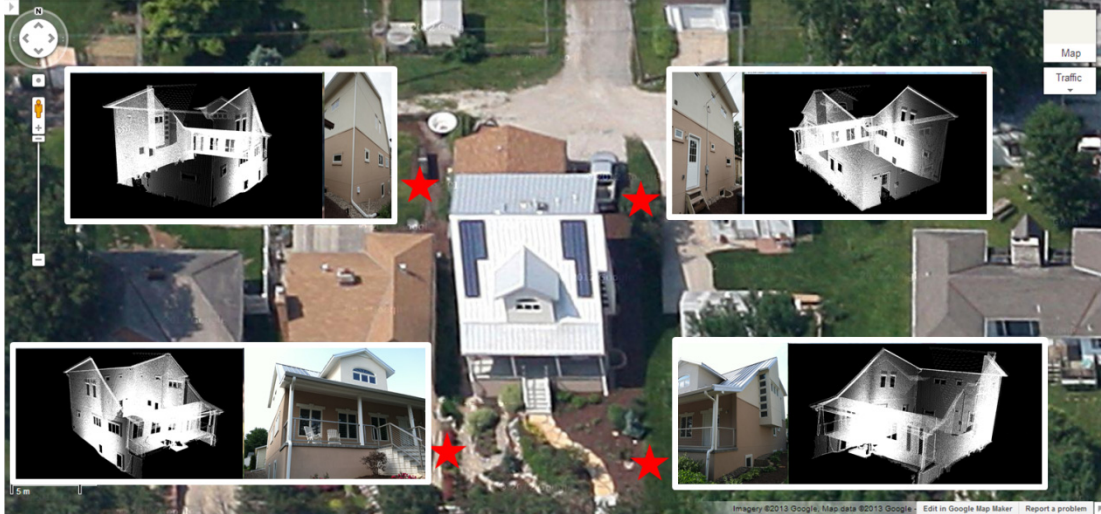
Figure 1. Collected point cloud of a residential house (stars indicate four locations of data collection)
