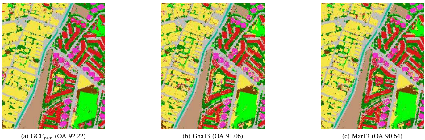
Fig. 6. Classification maps of Rome data set for the experiments reported in Table IV (standard deviation attribute): (a-b-c) \mathcal{P}_\rho + MS.
