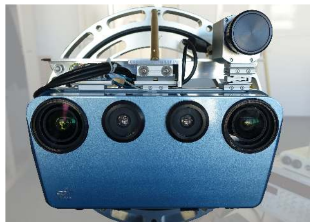
Figure 1. IPS Camera System with Optris PI 450 attached on top. The system is mounted on a rotary plate for calibration purposes.
