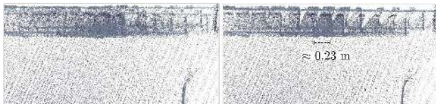
Figure 13: Detailed top view of the mail room scene shown in Fig. 12c. The top figure shows an uncalibrated sensor, while the bottom shows the calibration results. Protrusions going “inside” the wall are the mail boxes. Notice the expected more regular structure of the boxes post calibration.
