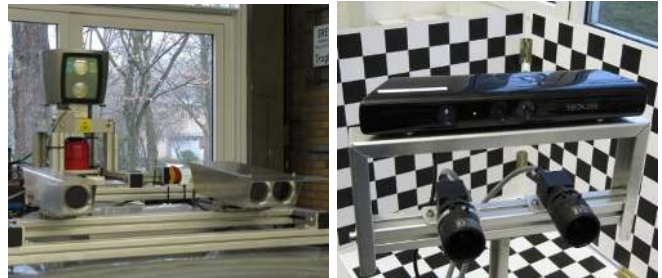
Fig. 1. Experimental setup. Trinocular camera with Velodyne HDL-64E laser scanner (left) and binocular camera with Microsoft Kinect (right).
