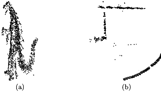
Fig. 7. Results: 3D point structure for the dinosaur sequence (a). The castle sequence (b) is shown in plan view with the estimated cameras.
