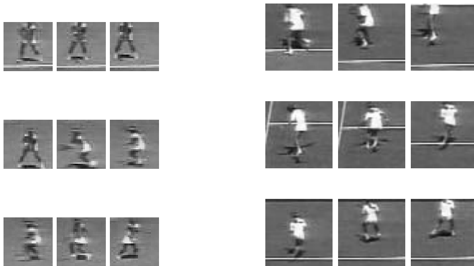
Figure 13: The templates of the players as they are tracked for 90 consecutive frames of the Passing-shot video segment. Shown on the left are the templates of the Top Player (TP), and those of the Bottom Player (BP) are shown on the right. The three rows of images correspond to the 3 successive chunks (each of 30 frames) in a top-down order. For each player, each row shows the templates etched out from the frames numbered 1, 15 and 29 in the corresponding chunk of 30 frames. The size of the TP templates is 30 \times 30 pixels and that of BP templates is 50 \times 50 pixels. The templates are shown at actual scale.
