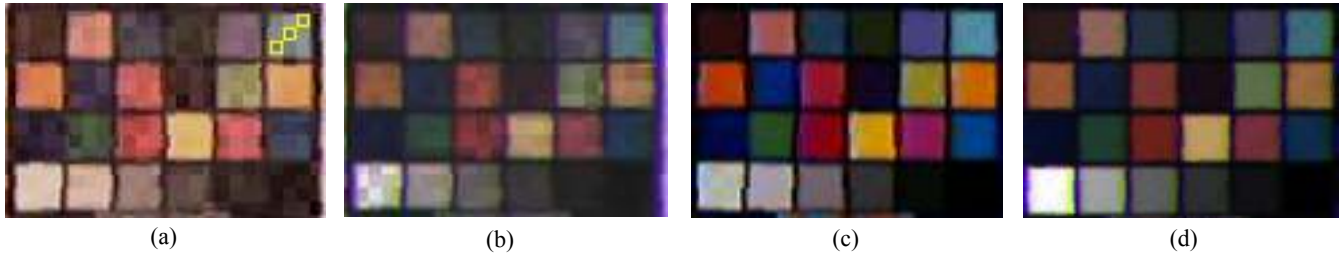
Figure 1: Image composites using blocks from different cameras. Blocks along a diagonal are from one camera. Three such blocks are highlighted in the first image. (a) Data from cameras at default gain and offset. (b) Cameras calibrated using software auto-gain and white-balance. Color inconsistency is significant. (c) Calibration of all cameras to a single standard - sRGB. Color artifacts are less perceptible although still noticeable in the white, yellow, and light green patches. (d) Our method, which calibrates cameras to each other, rather than to a standard. There are minimal artifacts. Note: Artifacts on the edges of color patches are due to demosaicing and geometric misalignment.
