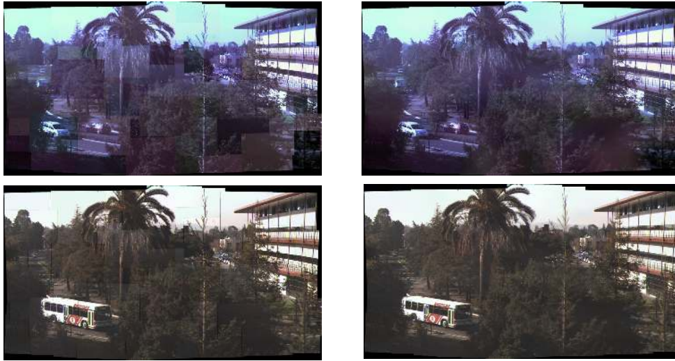
Figure 3: High-resolution image mosaics. Top Left: No color calibration and no blending. Top Right: With blending between images from each camera, the image seams disappear. Bottom Left: Using our method for gain and offset configuration, some image seams are visible, although they are not very harsh. Bottom Right: Blending between camera images removes the remaining seams.
