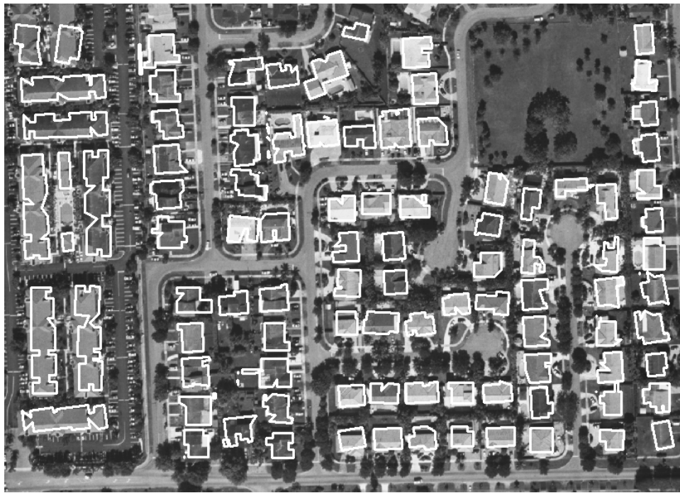
Fig. 11. Building footprints extracted from LIDAR data for a residential area.
