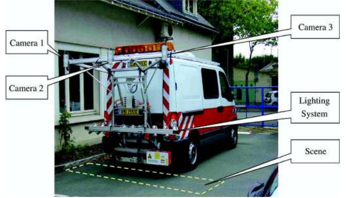
Fig. 4. Acquisition system used for the acquisition of the 38 images of data set 1: It is based on three sensors, and the processing is done 1\text{ m} \times 1\text{ m} with no overlap.
