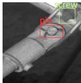
Fig. 10 Detection of the missing puller bolt by YOLO in Stage 2.
