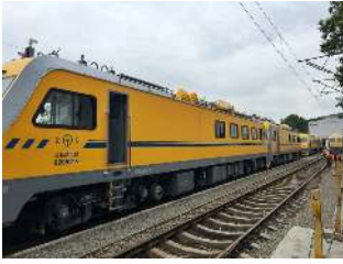
Fig. 12 XLN4C-01 inspection vehicle.
