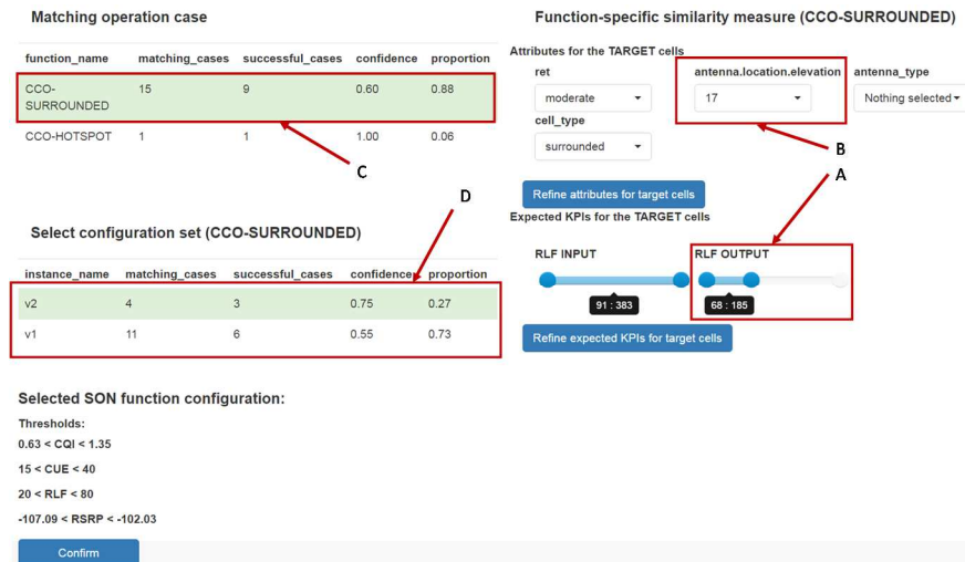
Fig. 7. A snapshot of the match result and configuration via refining the values of the function specific similarity measure.
