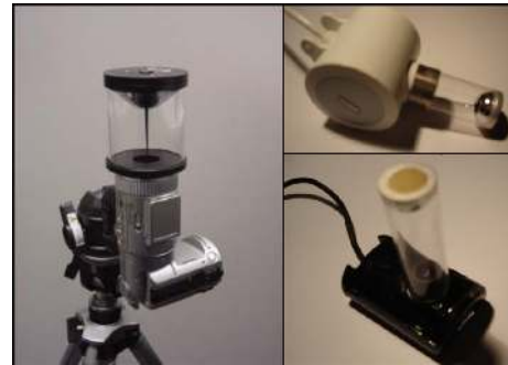
Fig. 1. Left: hyperbolic mirror placed on a video camera. Top right: Philips SPC 300. Bottom right: Philips ToUCam Fun.
