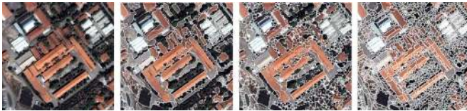
Fig. 12. Example segmentation results for the Ankara data set. From left to right: RGB color, result of the proposed approach, result of Pesaresi-Benediktsson, and result of watershed segmentation.
