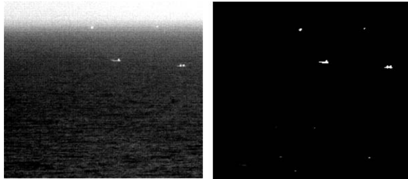
Figure 12: Detection of four small targets; two buoys, a zodiac and a 2-person kayak (zodiac and kayak at 1250 meter).
