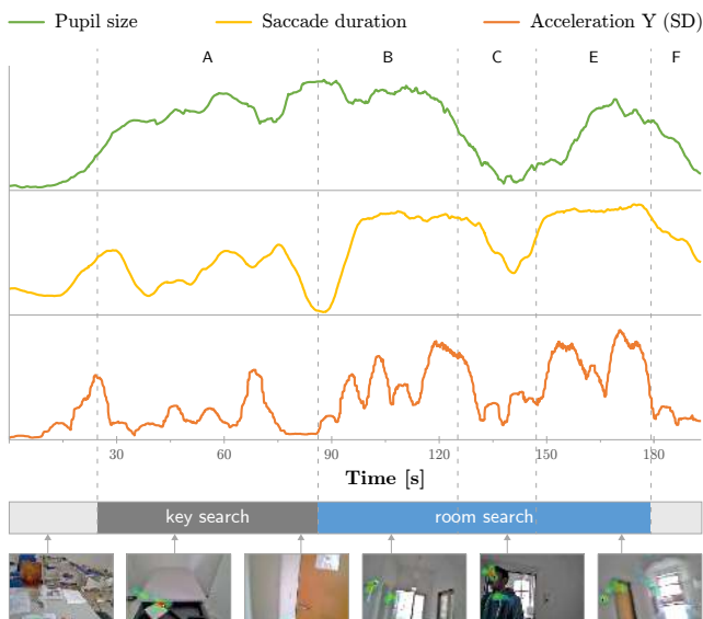
Fig. 8 Participant’s pupil size (mvavg over 8s, shifted left by 4s), saccade duration in a 4s window (mvavg over 4s) and SD of the accelerometer’s y-axis in a 4s window. Time Periods A-F as described in section 4.1
