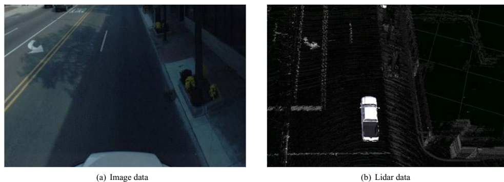
Figure 5. Counterexample showing that nonuniform lighting can play a critical role in influencing reflectivity/intensity correlation. (a) Ambient lit image with shadows of trees and buildings on the road. (b) Top view of the corresponding lidar reflectivity map, which is unaffected by ambient lighting due to its active lighting principle.
