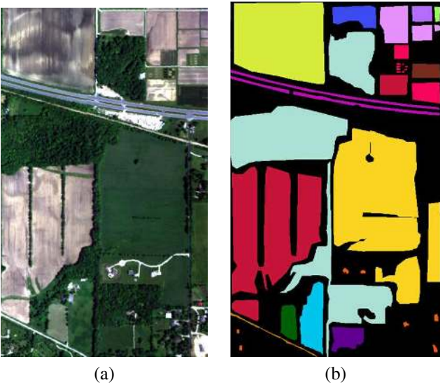
Fig. 3. Indian Pines 2010 SpecTIR data.(a) RGB composition and (b) ground truth. Color references are in Tab. II (unlabeled samples are in black).
