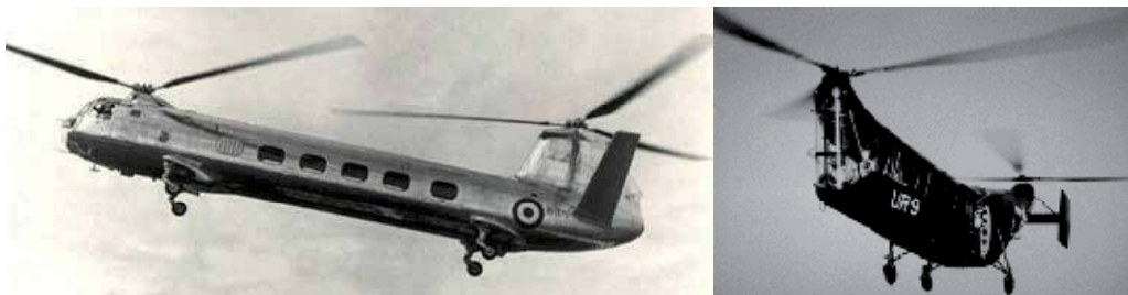
Fig. 2. Bristol 173 with cyclic pitch longitudinal control, Piasecki HRP-1 with differential pitch, www.aviastar.org
