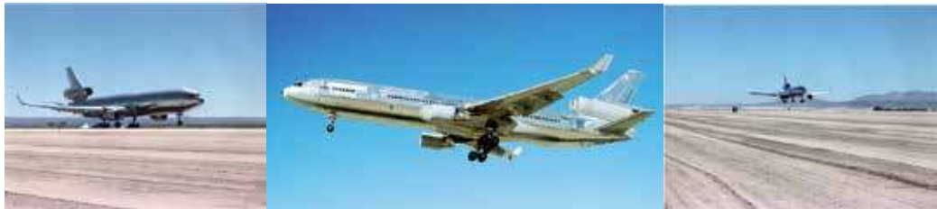
Fig. 1. McDonnell Douglas MD-11 landing at Dryden Flight Research Center equipped with a computer-assisted engine control landing system developed by NASA (NASA Dryden photo collection)
