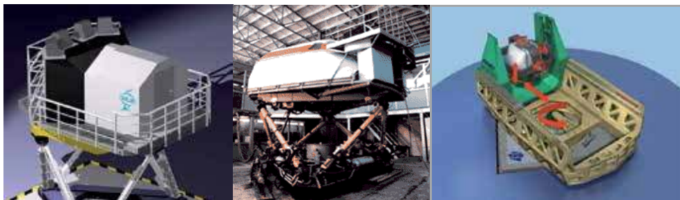
Fig. 16. SUPRA simulation facilities for conducting advanced upset recovery simulation research to improve pilot training in upset recovery and reduce LOC-I accident rates. Left: NLR Generic Research Aircraft Cockpit Environment (GRACE). Mid: TsAGI PSPK-102. Right: TNO/AMST Desdemona
