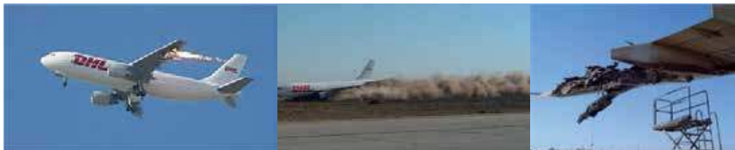
Fig. 2. Emergency landing sequence using engines only and left wing structural damage due to surface-to-air missile impact, DHL A300B4-203F, Baghdad, 2003
