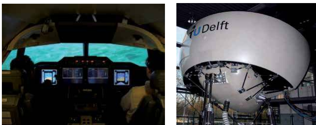
Fig. 12. Evaluation of GARTEUR FM-AG(16) FTFC techniques in the Delft University SIMONA Research Simulator based on reconstructed accident scenarios (Left: Boeing 747 cockpit configuration. Right: visual system dome)
