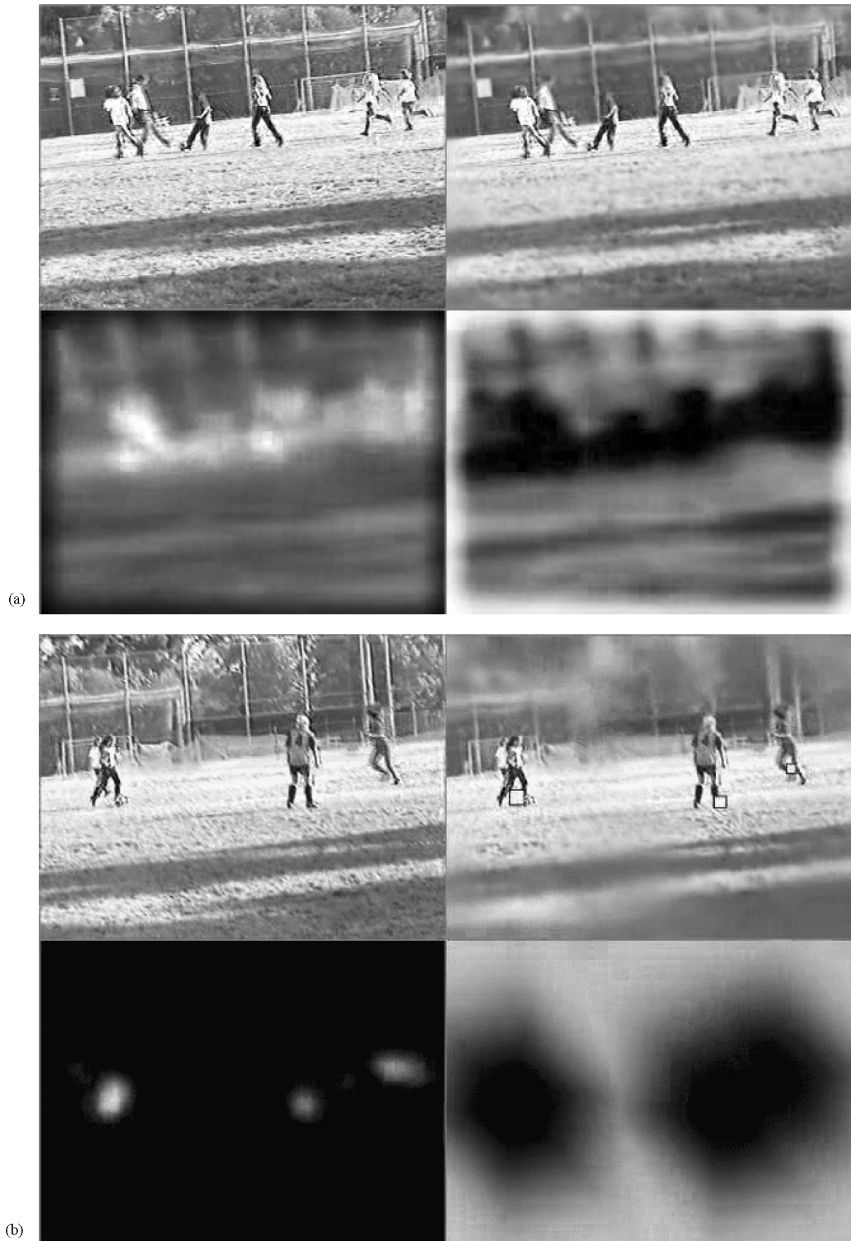
Fig. 2. Examples of predicted priority maps for two settings of our model. (a) Maxnorm feature normalization, continuous priority map (0 virtual foveas), foveation pyramid depth 4. (b) Fancynorm, three foveas, depth 6. Top left: original frame. Top right: foveated frame (with fovea centers marked by yellow squares when using discrete foveas). Bottom left: saliency map (brighter for higher saliency). Bottom right: priority map (darker for higher priority).
