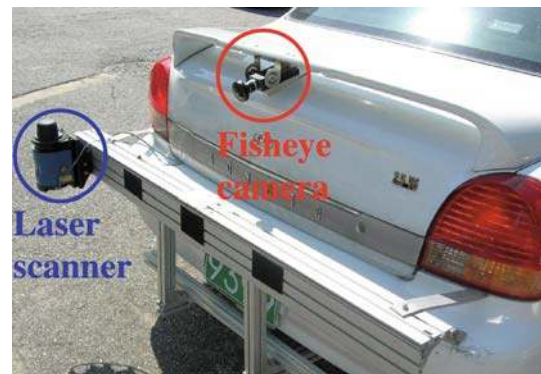
Fig. 12 Fisheye camera and laser scanner mounted on the automobile
