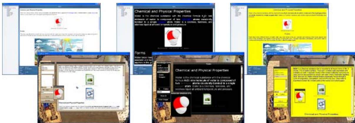
Figure 11. Adaptability of user interfaces for various visual disabilities. The leftmost pair of screenshots shows the default scheme (black text on a white background), whereas the pair in the center shows a scheme for visually impaired learners (white text on a black background, plus a 200% zoom factor). The rightmost pair of screenshots shows a scheme for colorblind learners (blue text on a yellow background).
