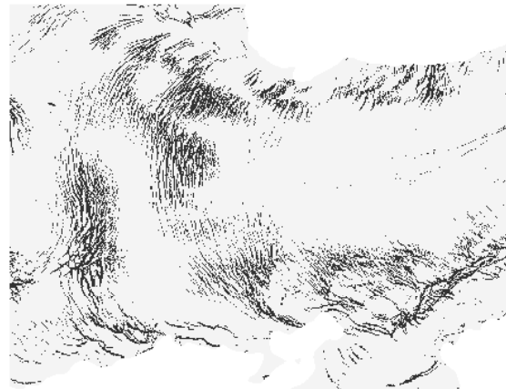
Figure 7. Detected crevasse locations.
