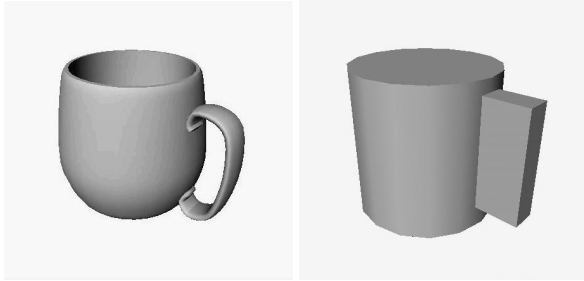
Figure 3: A mug model and its primitive representation. Because most mugs have a similar size and shape, this simplified model can be used for other mugs as well.
