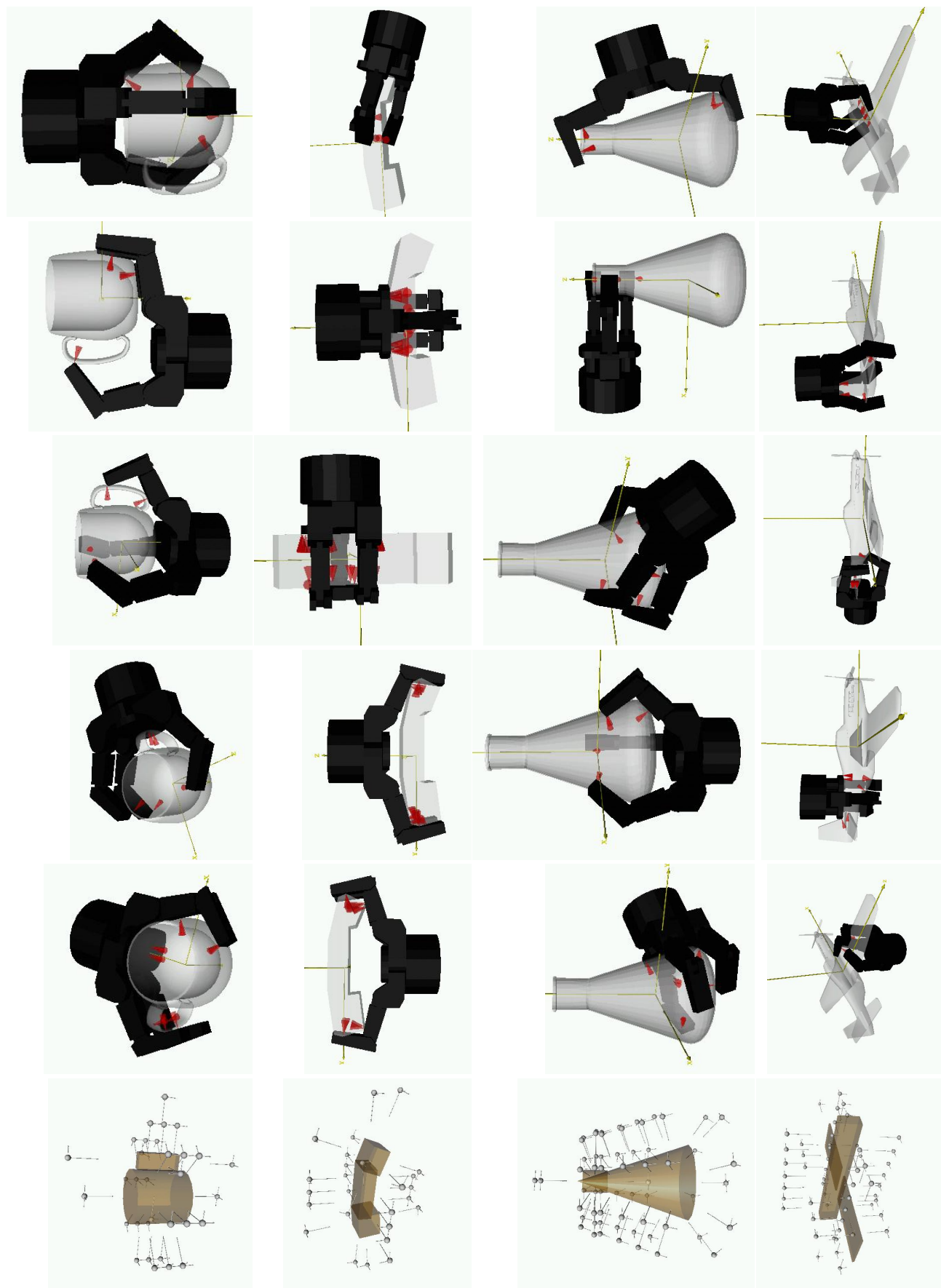
Figure 5: Planned grasps for a coffee mug, a phone handset, an Erlenmeyer flask, and a model airplane. The first image in each row shows the primitive model used for each object and the generated set of grasps to be tested. The other images show five of the best grasps found sorted in quality order.
