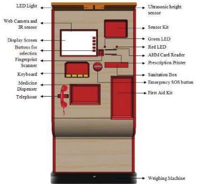
Fig. 4. Front view of the Automatic Health Machine
