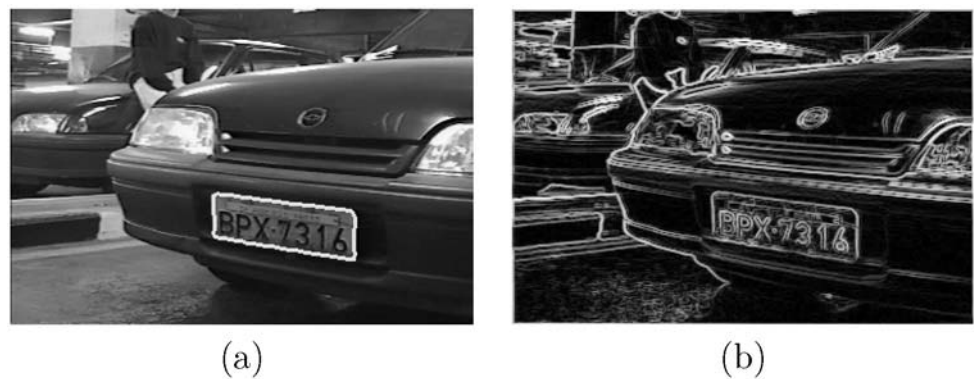
Fig. 13 a Original image with the result of TP. b The magnitude of the Sobel’s gradient
