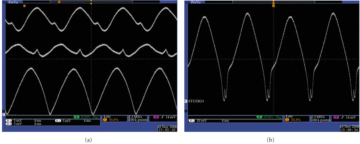
FIGURE 15: We depict the intensity output of various light sources. They do not follow a \sin^2 characteristic. Additionally, some light sources exhibit various distortions at the moments of on and off switching. In (a), three fluorescent lamps are presented, and in (b) the output of a Sox lamp is shown.
