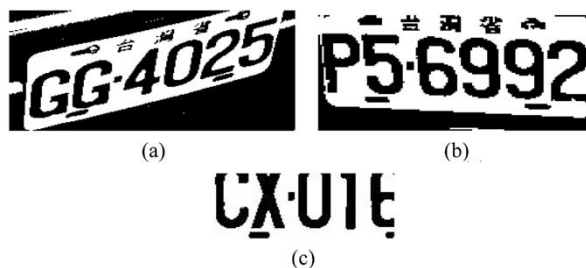
Fig. 14. Examples of imperfect license plate location: (a) skewed view, (b) over-segmentation, and (c) under-segmentation.
