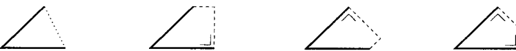
Fig. 3. If an edge hypothesis is not accepted, it is replaced by new ones. The dotted line is the original edge hypothesis, full lines are its (accepted) neighbours, dashed lines are the alternative edge hypotheses.
