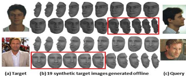
Figure 3. Examples of (a) original target face images, (b) synthetic target images generated offline using 3D face models, and (c) query images. The red rectangles indicate the online selection of synthetic target images based on the pose estimation from query images.
