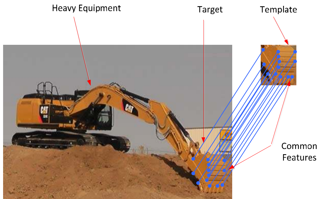
Figure 7. SURF features comparison between an equipment target and a template
