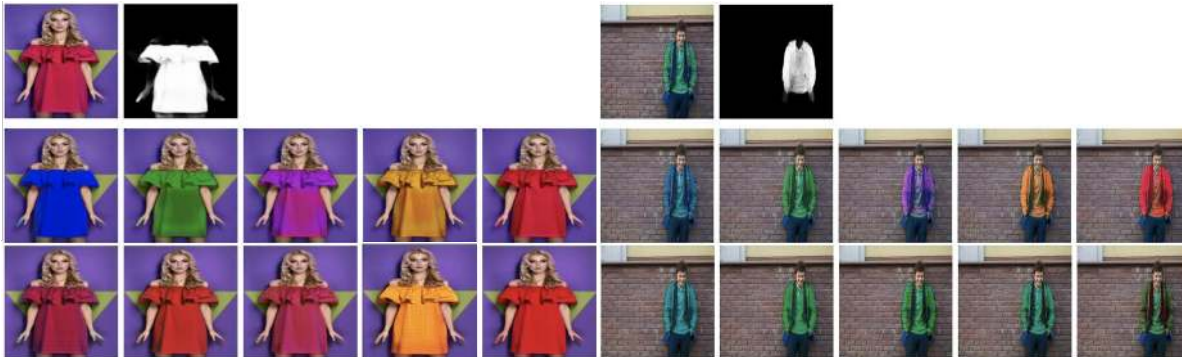
Figure 7. Top: Original image and mask. Middle: Paired discriminator. Bottom: Conditional discriminator. Recoloring to blue, green, purple, orange and red from left to right. We saw that during training on RGB images, a conditional discriminator is not able to generalize well and most of the time learns to generate just one particular color. Images are from FlexDreams - stock ID #112111227, romankosolapov - stock ID #111320345 .
