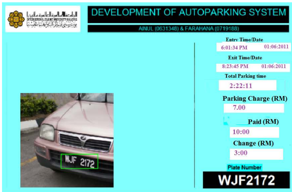
Fig. 7. Matlab GUI based car parking electronic billing window
