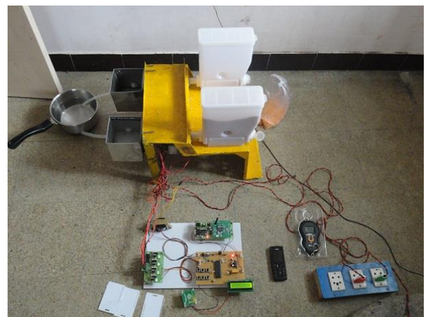
Fig. 9: Overall ration distribution system with mechanical parts
