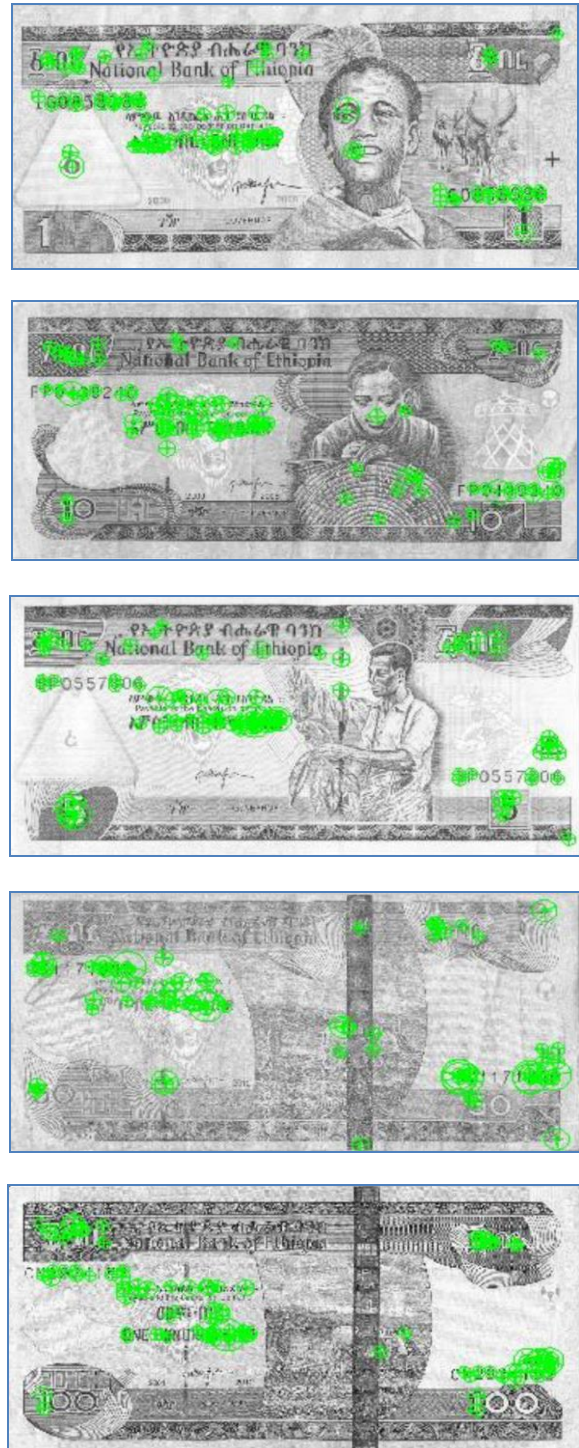
Fig.3. SURF points detected on Ethiopian banknotes (from top to bottom: 1, 5, 10, 50 and 100 Birr.)
