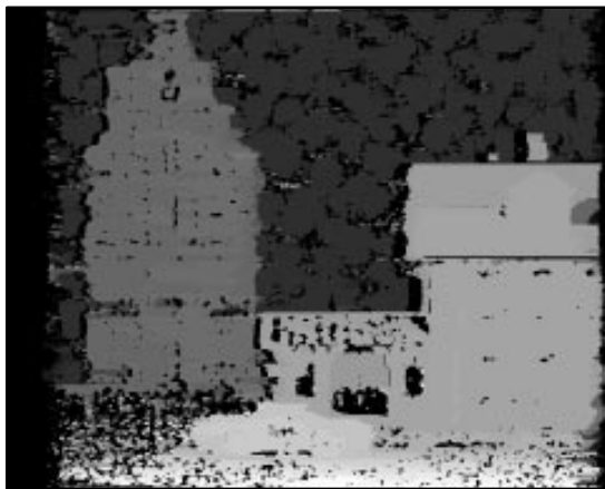
c) disparity map ( dark = far from camera, light = near to camera, black = undefined regions)
