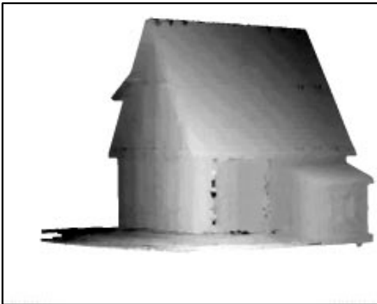
c) accumulated disparity map estimated from 9 adjacent image pairs, gaining sub pixel resolution
