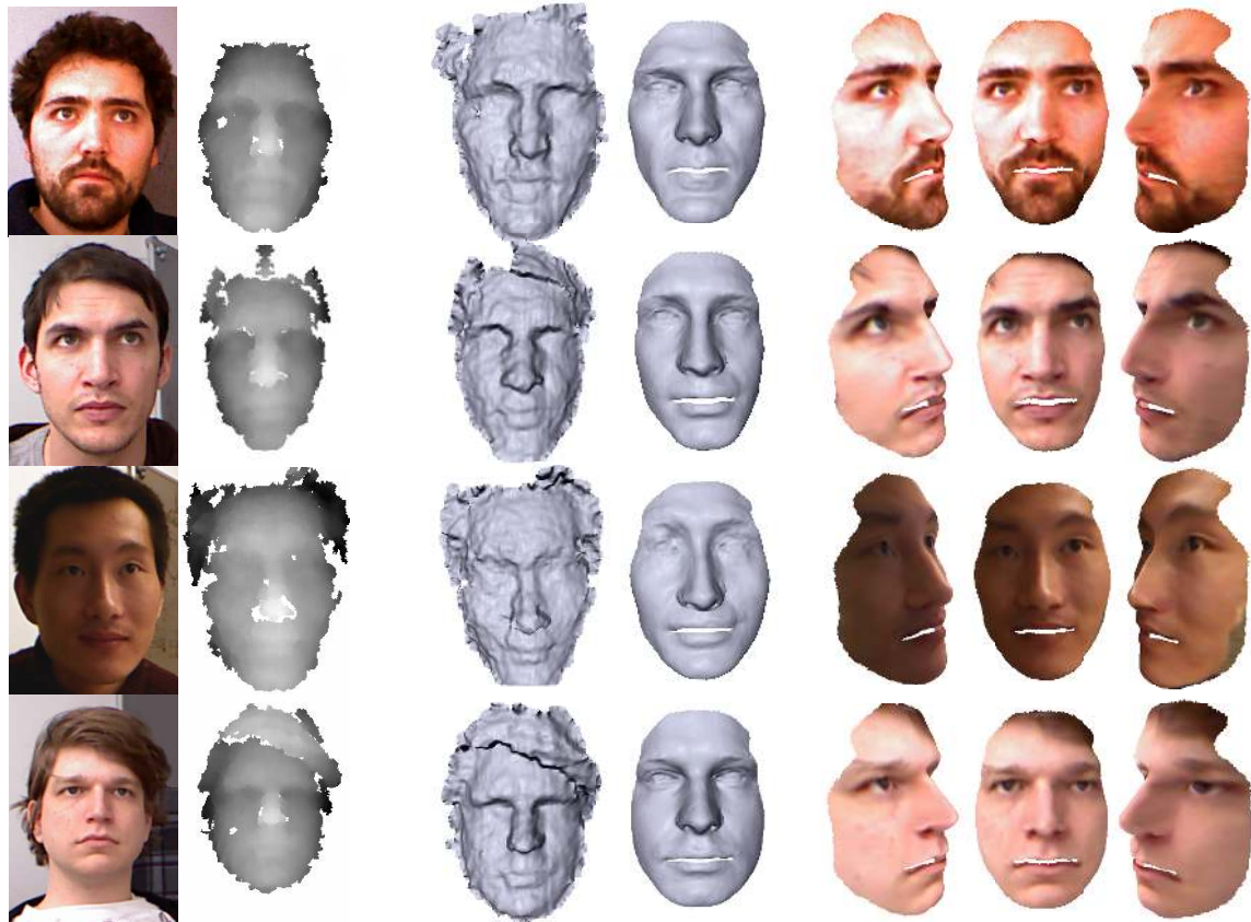
Figure 8: Face reconstruction results for four individuals. (from left to right) input RGB and depth images, processed depth scan, fitted face model and textured face from three different views.
