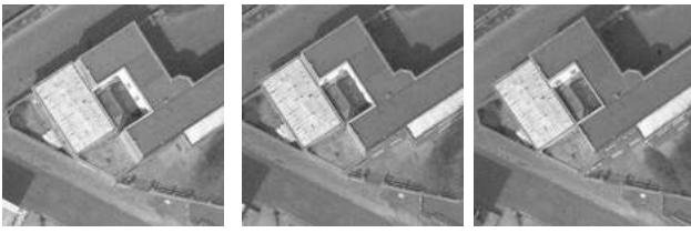
Figure 1. Three overlapping aerial views. The images are 600 \times 600 pixels, one pixel corresponding to a ground length of 8.5cm. The camera moves in a line at a height of 1300m, with about 300m between successive views.
