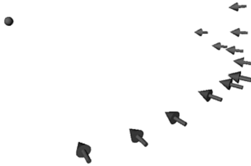
Figure 24: Estimated camera position and orientation for the 12 views of the Shoe sequence.
