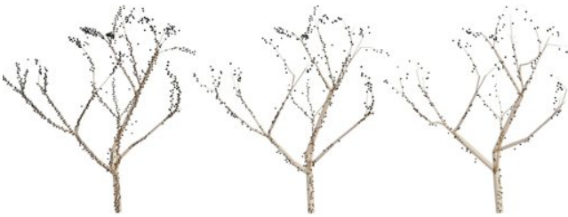
Figure 9: Robust tree reconstruction under varying point density. From left to right: the resulting BSG using 100%, 50%, and 25% of data points.
