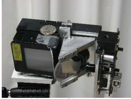
Figure 1: Texel camera constructed from a TOF depth sensor and an imaging (EO) sensor.
