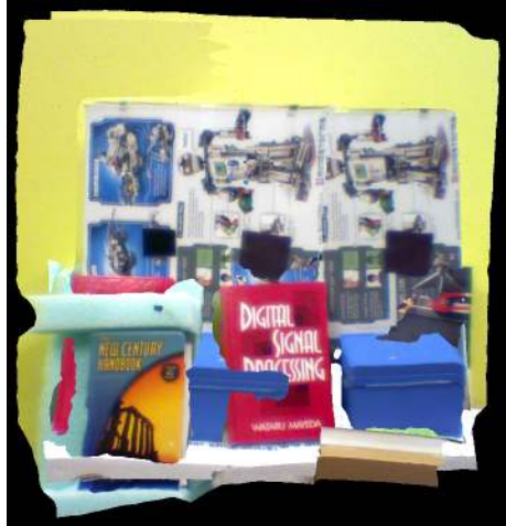
Figure 10: Registration result achieved using ICP on the lidar point cloud only.
