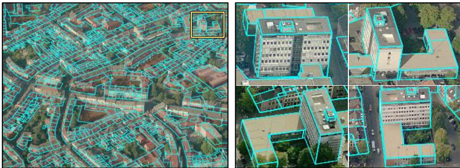
Fig. 7. Left: Registration result for one out of 36 images ( 3 \times 3 for each cardinal direction) of an urban area. Right: Projection of a 3D building model into 4 images (out of 11 in which it is visible) to verify the precision of the automatically obtained registrations. The projections of the model are aligned with the images with only minor deviations of at most 1-2 pixels, which translates into a maximal positional imprecision of 15-30cm in scene space.
