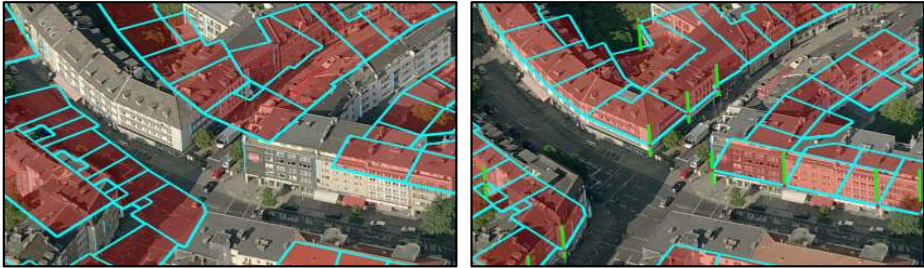
Fig. 4. Result of the initial registration process. Starting from a rough estimate of the registration parameters (left), our system automatically recovers good initial registrations for each individual image (right). Vertical line constraints are shown in green.
