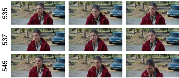
Figure 3: Each row shows the first, middle and last frames in a thread of shots from ‘Love Actually’. The colour histogram difference between the last frame of shot 535 (top) and the starting frame of shot 537 (middle) is greater than that to the starting frame of shot 545 (bottom), because of small lighting changes in the background which change the histogram (though this is hard to perceive by eye). However, in order to find continuity errors, it is important that the middle shot is matched, as this is the shot which comes from a different take to the majority of other shots in this thread.
