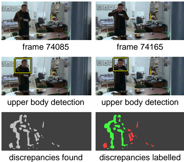
Figure 5: The steps of the spot-the-difference process. Top row: two initial frames. Middle row: Upper body detections in each frame. Bottom left: Thresholded differences found between the two frames after registration. Bottom right: differences classed as either potential error (red) or as a discrepancy due to a person (green).
