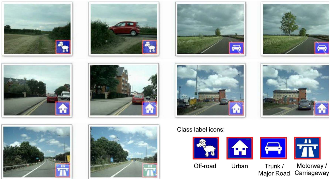
Fig. 4. Examples of successful ANN classification for four road environments (ANN configuration: H = 15 Nodes; I = 200 ).
