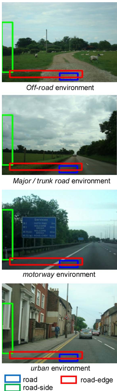
Fig. 1. Subregions of interest selected for feature extraction for the four road environments under consideration.
