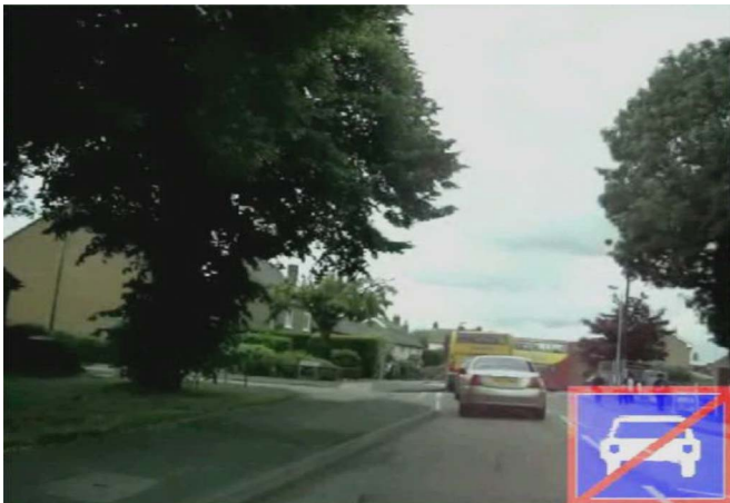
Fig. 8. Misclassification as “off-road” instead of “on-road.”
