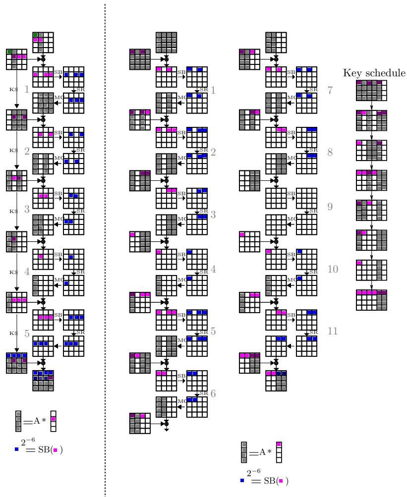
Fig. 2. The best characteristics for AES-128(left) and AES-192(right). The first one is on 5 rounds, while the second one is on 11 rounds.
