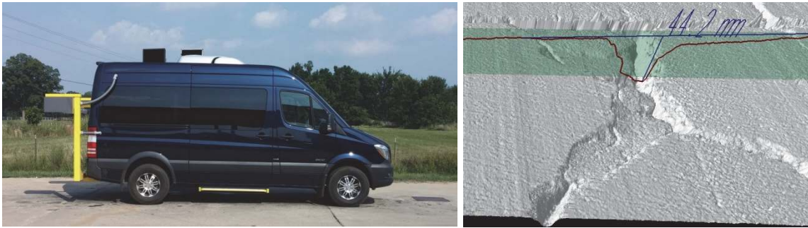
FIGURE 2: PaveVision3D Ultra System (left) and representative 3D pavement data (right).
