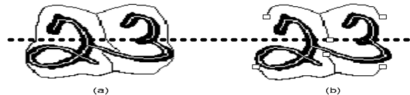
Figure 5: (a) Original top / bottom-background-skeletons. (b) Top / Bottom-background-skeletons after removing parts which are lower/higher than the middle line (Horizontal dashed line is the middle line, which divides the image into two parts with equal heights).
