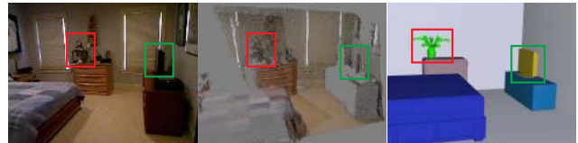
Figure 16: Higher \lambda_c helps recover objects with lower classification confidence (e.g. the TV set), but causes misidentification of point clouds that should be rejected by the classifiers (e.g. the plants).
