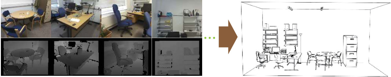
Figure 1: Automatic semantic modeling of an office scene. Left: input RGB-D images, right: reconstructed 3D scene.
